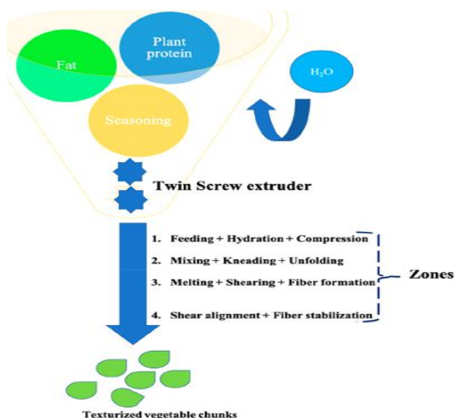
Fig. 2 : Extrusion technique of making texturized plant-based meat analogues (Arora et al. , 2020).
